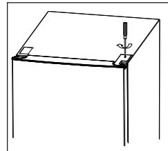
2. Unscrew and remove the hinge.
