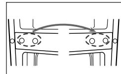
5. Unscrew bottom hinge. Then remove the adjustable feet from both side.
