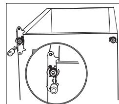
8. Make the middle hinge reverse the direction 180°, the transfer it to the left property position. Make the middle hinge pin in the upper hole of the lower door, then tight the bolts.
