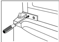
9. Place the upper door back on. Ensure the door is aligned horizontally and vertically so that the seal are closed on all sides before finally tightening the top hinge. Then inert the hinge and screw into the front of the unit.
