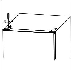
13. Fix the hinge cover on the left and the hinge hole cover on the right.
