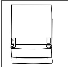
10. Unscrew the hinge pin and reverse the hinge, then reinstall the hinge pin.
