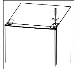
3. Unscrew middle hinge. Then lift lower door and place it on a soft pad to avoid scratch.
