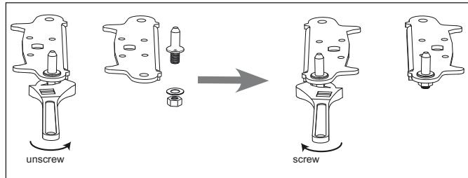
7. Refit the bracket fitting the bottom hinge pin. Replace both adjustable feet. Transfer the lower door to the property position.
